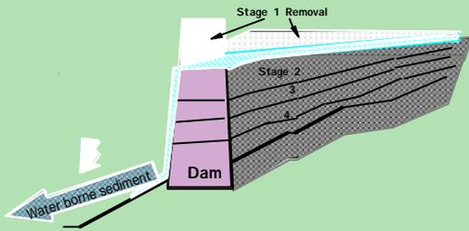
Remove dam in phases and allow sediment to transport naturally, in stages
