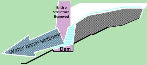
Complete removal of dam, allowing natural transport
