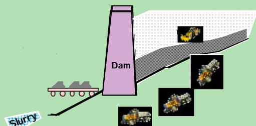
Move sediment downstream by trucking, slurry, or conveyor
